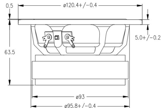
The W12CY002 is a 12cm (4,5") cone driver developed for use as a high fidelity woofer/midrange unit. The extremely stiff, yet light cone gives tremendous bass precision and midrange detail.
