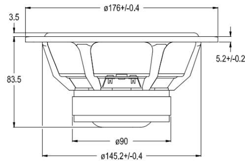
The W18E001 is a 6,5" cone driver developed for use as a high fidelity Woofer or Woofer/Midrange unit. The extremely stiff, yet light cone and the acoustically transparent basket give tremendous bass precision and midrange detail.
