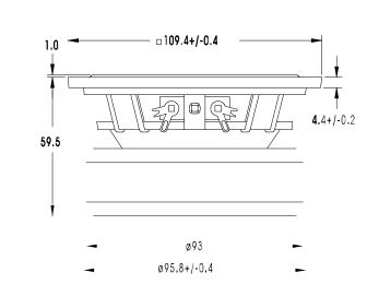
CA11RCY, (11 F-GX) is a 4.5" High Fidelity mini woofer with a stiff and stable injection moulded metal chassis. A natural rubber surround and handcoated paper cone with coated fabric dust cap, reduce resonances and distortion. Excellent linearity is achieved with a large magnet system and a symmetrical driving force accomplished with a special winding technique for the voice coil. A very large magnet system provides a reasonable efficiency and a low Q.
